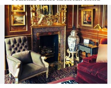
Polished Brass Register with punch-marked engraving, roundels and plinths on front surround. Incorporating spark mesh curtains with fire enclosure and solid brass front basket with urn finials uppermost
